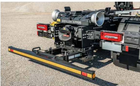
Hydraulic underrun protection
