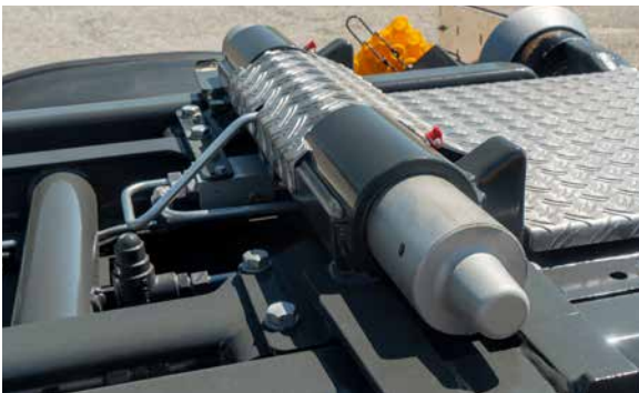
Hydraulic skip locking system
